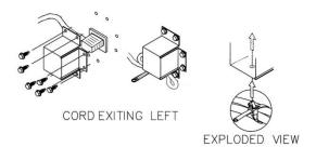
Figure 8.2 Power Cord and Protective Cover
