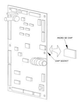
Figure 8.1 Loading Control Software
