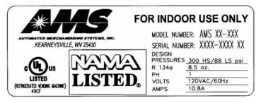
Figure 1. Example of Serial Plate
